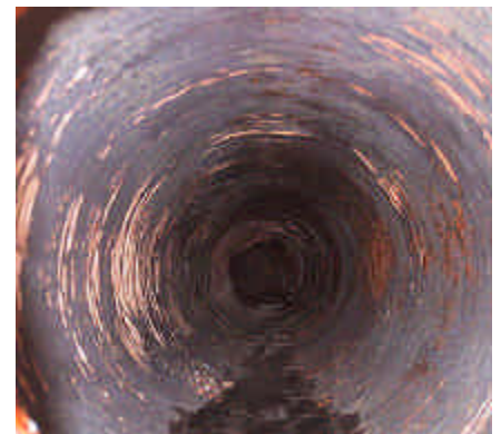
Heavily contaminated pipes blasted to smooth finish by tank cleaning head.
