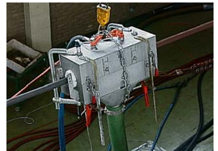
Decontaminating coiled tubing
